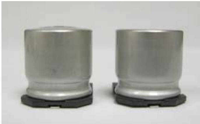
Figure 1: Aluminum liquid electrolytic capacitor, on the left-hand side, that has experienced case distortion after an extended time at Pb-free reflow temperatures
